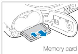
Push the card gently until the card disengages from the camera, and then pull it out of the slot.
